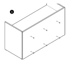
2 Align Overlay Panel and drive Bolts into threaded inserts to hold in place.
