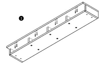
Slide Panel onto posts and tighten Cams, access thru paper slot opening, as shown.
