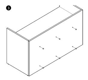
Center Paper Slot unit and drive 15/8" Screws into Panel to hold in place.
